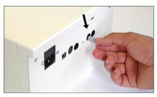
2 Use a flathead screwdriver to secure each connection. Do not overtighten.
